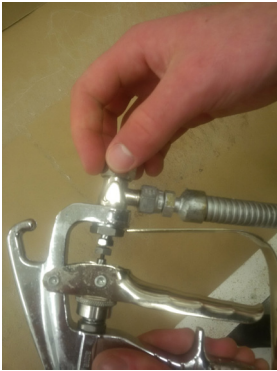
1. Unscrew tip retainer
