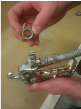
4. Lay tip retainer on top
