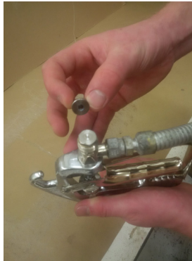
2. Lay spray tip on top
