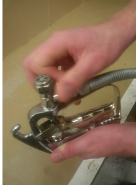
5. Screw on tip retainer
