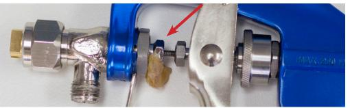
The adhesive only passes through a very small part of the gun when being sprayed. To prevent the adhesive from leaking out of this area, it is sealed off. This seal is held in place by a nut. Over time, this can become loose, causing the seal to fall out of place. This needs to be tightened. However, be careful not to make this to tight, as it will cause the sliding pin to bind and the trigger will become stiff.
