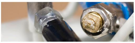
Over time, the gun tips can build up with dried adhesive. When this happens, the gun can't close off properly, so the adhesive continues to dribble out after the trigger is released. To fix this, simply remove the gun tip and clean with TensorGrip C101. In extreme cases, a replacement tip may be required.
