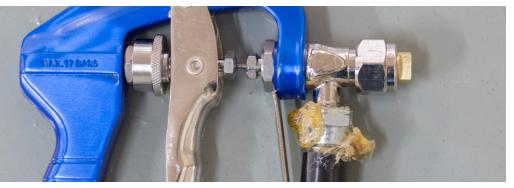
If so, it is too loose and needs tightening. The gun and hose are designed to join almost seamlessly together. This is to provide the adhesive with a straight, unbroken trajectory to the gun tip. Any breaks or gaps in this line will mean the adhesive will leak out.
