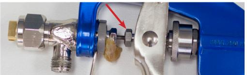
Ensure the nut on the opposite end of the threaded rod is finger tight against the gun trigger. This will allow the pin to move freely to release the adhesive. Do not tighten this screw with a spanner as this will break the pin and your gun will need replacement.
